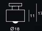
SNOWFLAKE W SQ-2757WF E27 1 x Max 40W Crown mouth-blown glass, steel Canopy: A6 Plate: B
