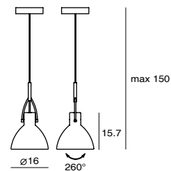
LAITO P S SQ-895MP E27 1 x Max 46W Halogen matt black/ matt pure white/ chrome/ copper shade rotatable Canopy: A Plate: A
